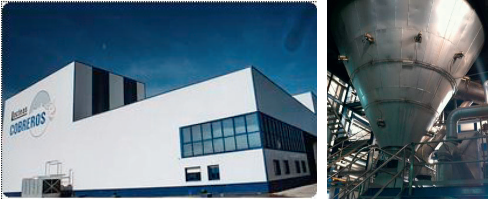
Fig. 5. Production site at Lácteos Cobreros S. A. (Picture right: milk drying cyclone)
