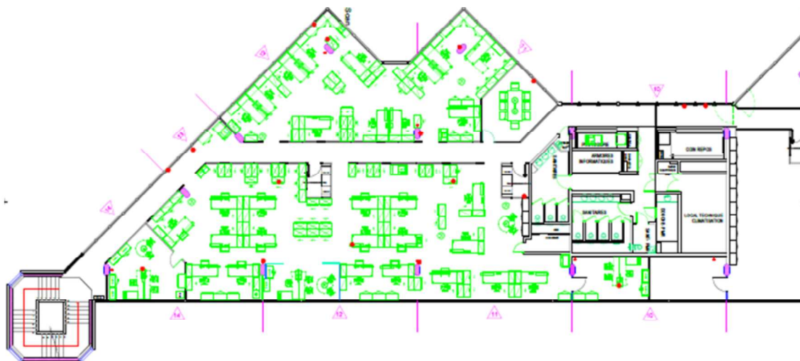
Figure 2: Installation plan of BuildAX sensors (the locations of the sensors are marked with a red dot).
