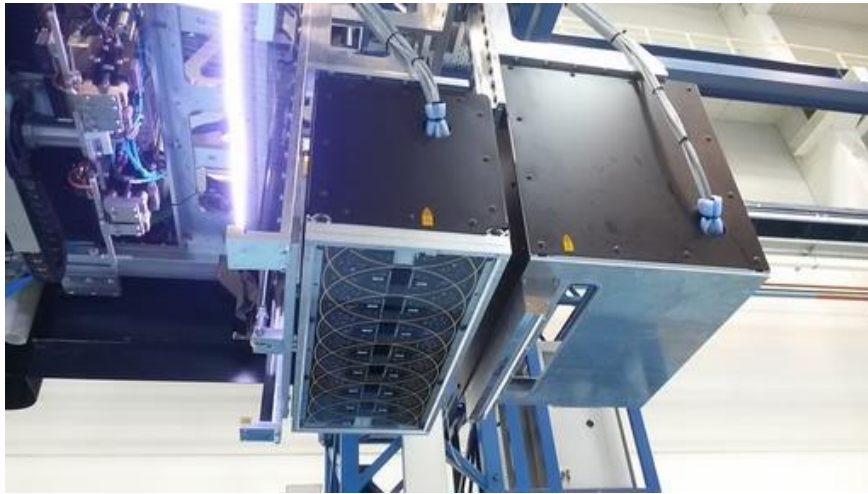
Figure 3. Integration of the sensors into the placement head. The fibre orientation sensor is in the center of the image with the characteristic LED light rings and the laser profile scanner is mounted to the right.
