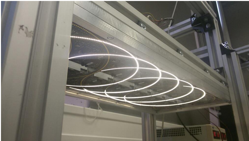
Figure 2. Each sensor module uses a ring of LEDs. The single rings overlap to allow an arrangement of the sensors in a single row. Switching of the LED modules is arranged so that sensors do not interfere with each other.
