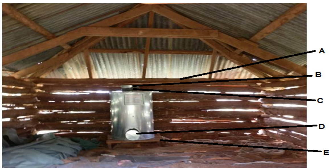
Figure 2. The adoption of the small scale metal silo in grain storage instead of the wooden crib (A) can be a great step in reducing post harvest losses of grains in sub-Saharan region. The metal silo usually has one grain inlet (B) which is secured with a rubber band (C) and an outlet (D). The metal silo is usually placed on a wooden pallet (E) to keep it cool.
