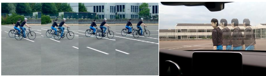
Figure 5 - Examples of advanced dummy features: Pedaling cyclist dummy with rotating wheels (left)
