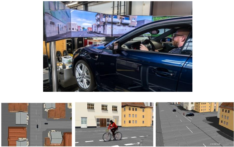
Figure 4 - Audi Mobile driving simulator presentation Two additional monitors mounted (above) Driver and VRU perspective (below)
