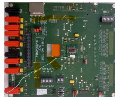
Fig. 6. Radiation Test Board designed for the XCZU3EG Device, with one de-lidded device.
