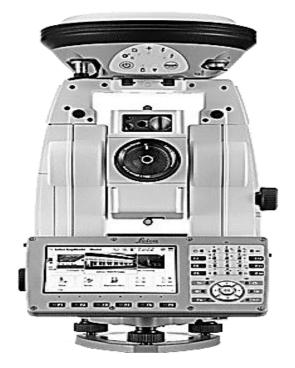
Figure 1 Integrated Total Station and GPS
