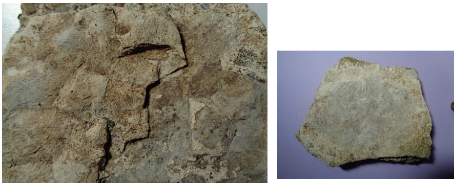
F31 B. Detail of the course part of the mortar: large inclusions of lime glued together. The structure of the mortar gets more fine tempered to the outside, till a smooth surface has been realized to form the plaster. The image right shows a slight difference in color at the surface, showing an horizontal oval shaped discoloration, probably due to original painting.
