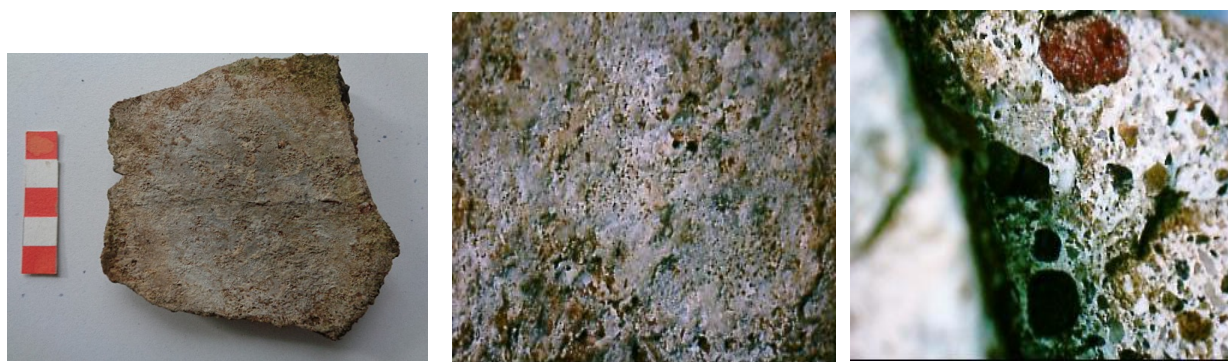
F 30. Fragment of Roman plaster with mortar, most likely a wall fragment (left). Middle: surface of plaster (probably the wall surface) detail (magnification 3 x); right detail of mortar consisting of lime, recycled pottery and lithic fragments,
