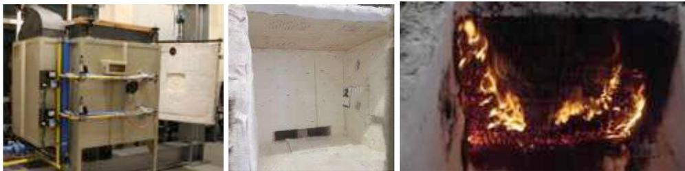
Figure 3 – Fire resistance furnace in laboratory, before and after the test
