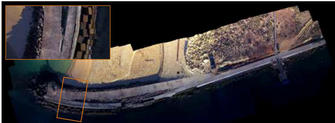
Figure 11 – Orthomosaic (with detail) of the west breakwater of Faro-Olhão for drone campaign of July 25<sup>th</sup> 2018
