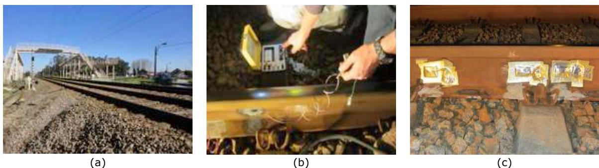
Figure 1 – (a): Location of Estarreja test site, North view, (b): strain gauges installation, (c): strain gauges installed on the rail web
