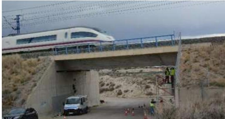
Figure 13. Placing the accelerometers
