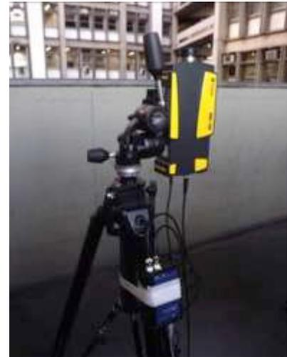
Figura 8 - Ensaio 2: Vibrômetro a laser Polytec (Portable Digital Vibrometer: PDV-100)
