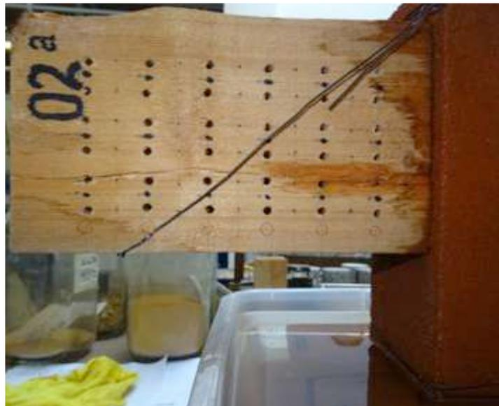
Figures 8 and 9 – Four edge corners of the face (e) getting wet (left), and superficial moisture spreading along the grain on the face (a) at the timber beam-end in contact with wet masonry (right), from Tola (2017).
