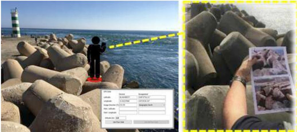
Figure 4 – Visual observation technique used in the Faro-Olhão's east breakwater
