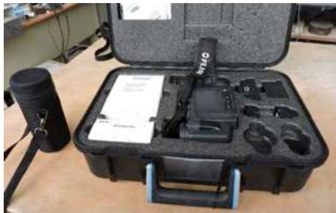
Figures 3 and 4 – Moisture meter (left) and IR-thermographic camera (right), from Tola (2017).
