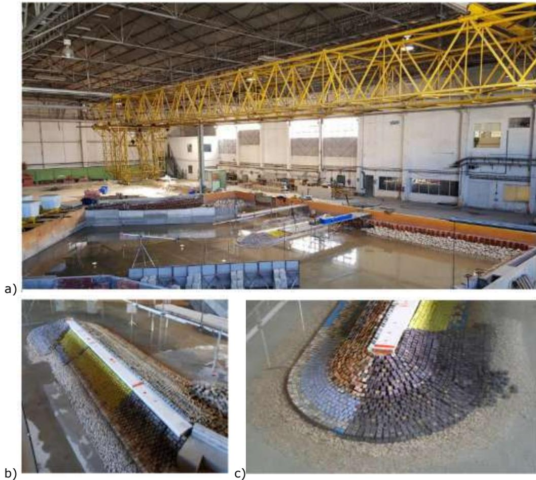
Figure 5 - a) Overview of the irregular wave tank b) Three-dimensional scale model c) Detail of the breakwater's roundhead
