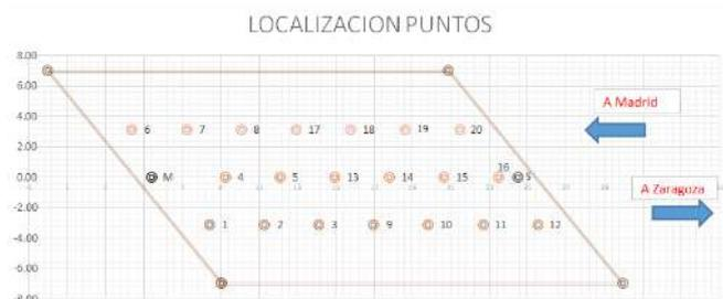
Figure 12. Accelerometers distribution
