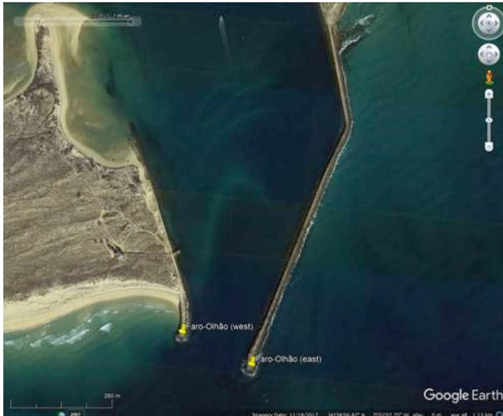
Figure 2 – The east and west breakwaters of Faro’s harbour entrance, in the protected area of Ria Formosa
