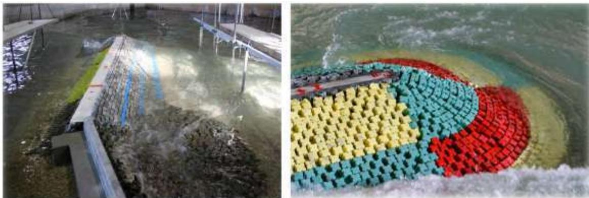
Figure 2 - Examples of three-dimensional stability scale model tests
