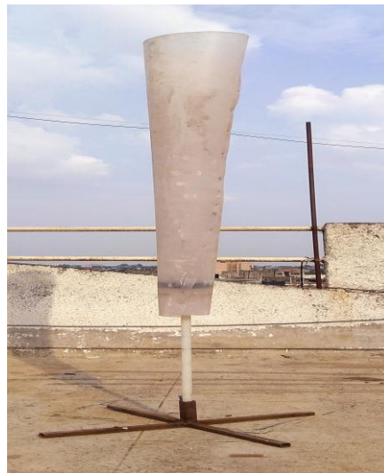
Figure 11: Vortex bladeless windmill.
