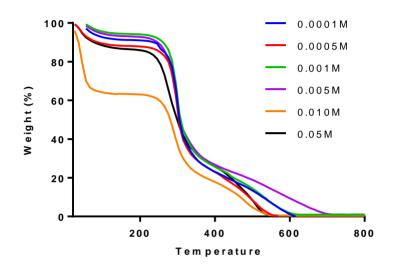
Fig.3 TGA analysis of CDS at variable concentrations of Na<sub>2</sub>CO<sub>3</sub>
