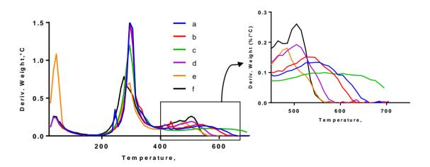
Fig4.Comparison of DTG of CDS samples at variable Na<sub>2</sub>CO<sub>3</sub> concentration
