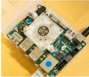
Figure 1: Odroid XU3 used to execute uploaded CMB programs. It is available at <https://climb.idi.ntnu.no> through a graphical user interface. It contains a modern heterogeneous processor typical for recent smart phones. The user select from a menu of programming problems and submissions are ranked according to execution time or energy efficiency.
