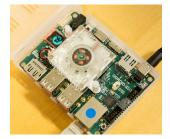
Figure 1: Odroid XU3 used to execute uploaded CMB programs. It is available at https://climb. idi.ntnu.no through a graphical user interface. It contains a modern heterogeneous processor typical for recent smart phones. The user select from a menu of programming problems and submissions are ranked according to execution time or energy efficiency.
