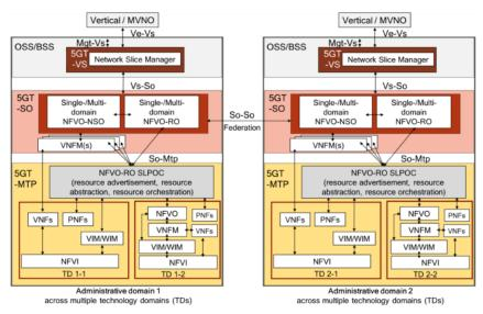
Figure A-1: 5G-TRANSFORMER system architecture [97]
