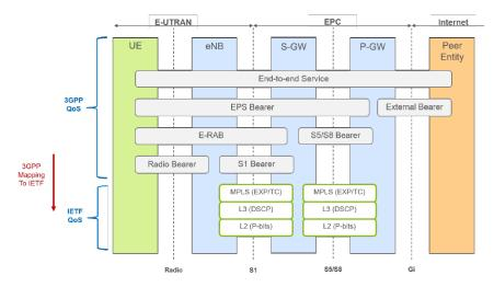
Figure 4-2: E2E QoS design uses a blend of the 3GPP and IETF QoS architectures
