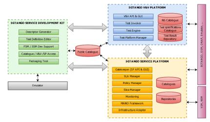
Figure A-3: Overall 5GTANGO architecture [101]
