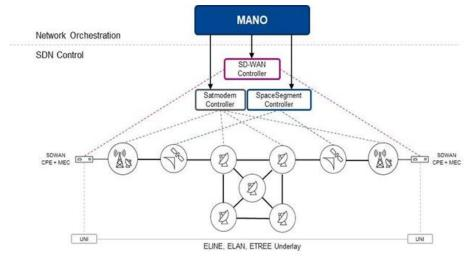
Figure 4-21: Distributed SDN Controller Architecture [77]
