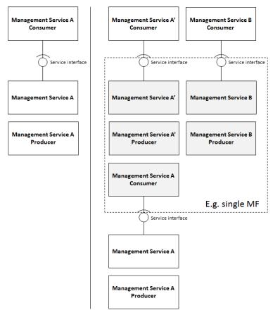
Figure 5-1: Exposure as conceptualized in item 4.4 of TS28.533 in 3GPP SA5 [49]
