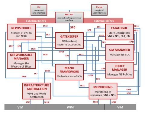
Figure 2-11: SONATA Service Platform Architecture [36]
