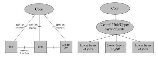
Figure 4-11: Non-centralized vs. centralized RAN deployment [57]
