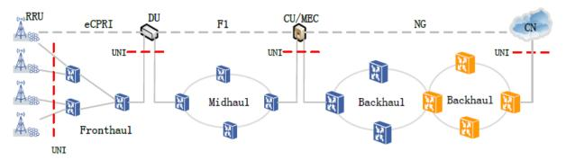
Figure 4-12: Transport network architecture for independent CU and DU deployment [56]
