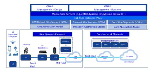
Figure 2-12: 5G network slice - network architecture with ONAP management [38]
