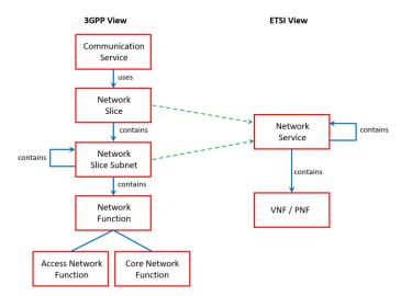
Figure 2-3: Relating 3GPP and ETSI models in the context of network slicing [20]
