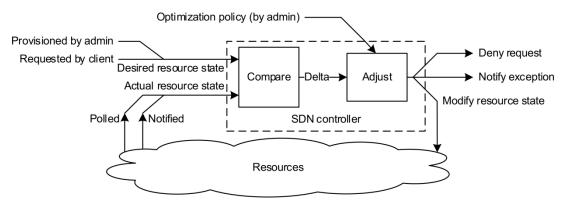
Figure 5-4: Control as feedback [80]
