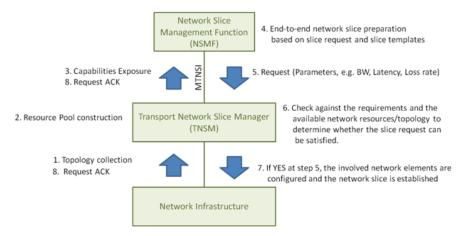
Figure 4-10: NSMF - TNSM mapping procedures
