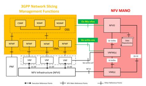
Figure 2-5: 3GPP network slicing management in NFV framework (adapted from [20])
