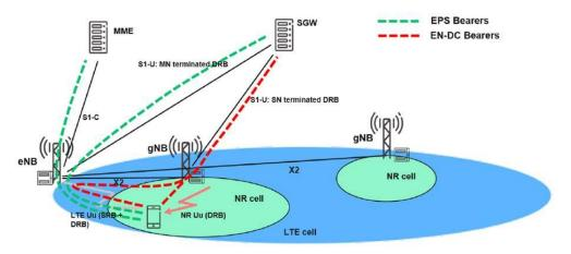
Figure 4-3: Conceptual Architecture for EPS with EN-DC (Option 3x)
