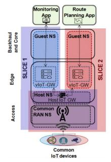
Figure 6-2: Extended mMTC Slicing Model
