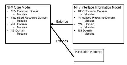
Figure 5-8: NFV Core Model extensions
