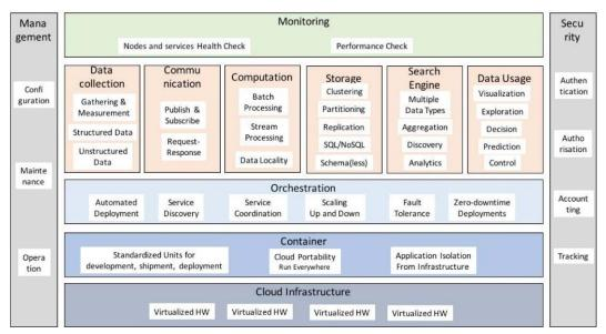
Figure 2-7: A High-Level Architecture for IoT Virtualization [26]
