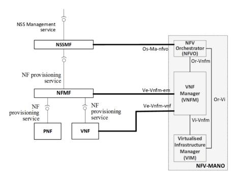
Figure 3-5: Example of 3GPP ETSI NFV interaction from TS 28.533 [49]
