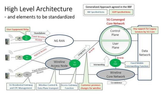
Figure 4-6: BBF 5G FMC architecture and elements to be standardized [55]
