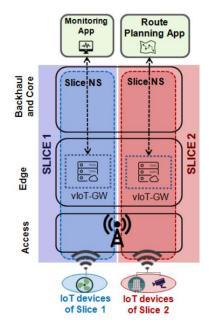
Figure 6-1: Baseline mMTC Slicing Model
