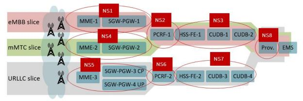
Figure 3-4: Composition of Network Slices based on Network Services
