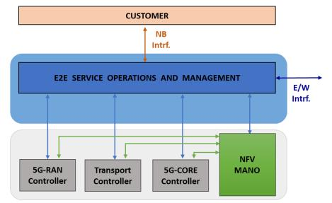
Figure 3-1: Architectural Components for the slice life cycle management and orchestration
