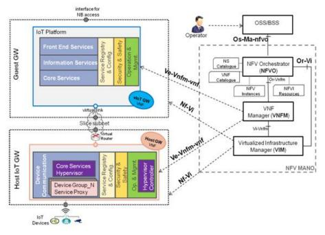
Figure 6-3: Interfaces for mMTC slice lifecycle management
