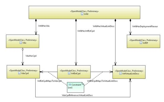
Figure 5-9: VNFD High-level structure
