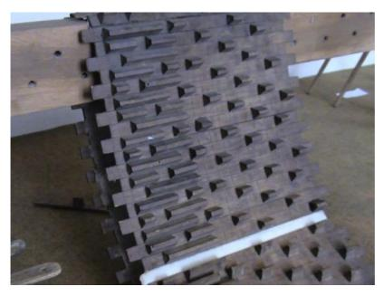
5 Detail of the pattern input strip for the crumb-maschine in the Weaving Museum Haslach. Wooden strips and pegs are glued onto the linen band. One peg is lost and the linen is visible. Photo Ellen Harlizius-Klück.
