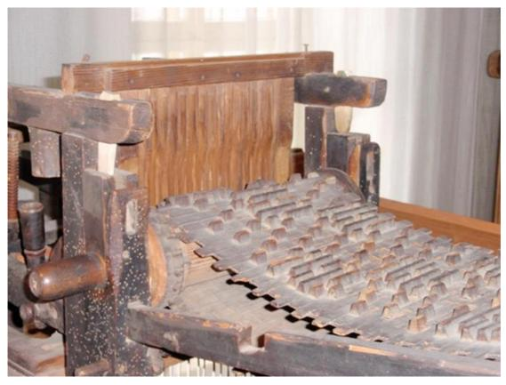
4 Detail of crumb-maschine with cylinder and vertical hooks. Photo Ellen Harlizius-Klück.
