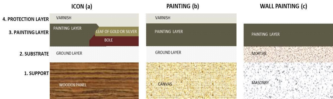
Figure 1. Painting artwork construction materials for (a) portable icons with egg tempera technique on wooden panel, (b) oil paintings on canvas and (c) wall paintings i.e. fresco or secco.
