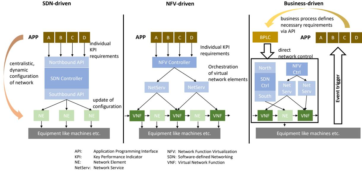
Fig. 2. Comparison of SDN- and NFV-driven network management to the BPLC approach
