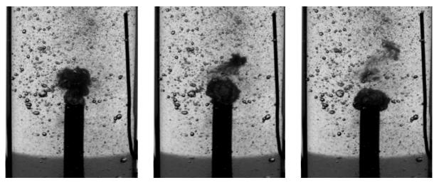
Figure 4: Example of the evolution of the growth and collapse of steam bubbles during CHUG experimental test, as recorded by the high speed camera.  $t^*$  is an arbitrary time instant when the steam-water is still contained inside the injection nozzle.
