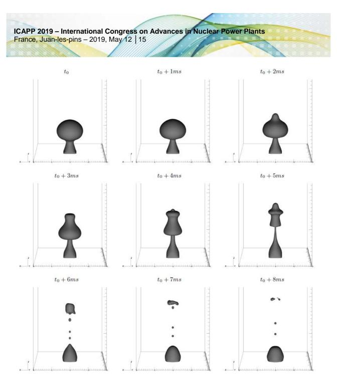
Figure 6: Example of the evolution of the growth and inertial collapse of a steam bubble, as simulated by PSI-BOIL [4].*t*<sub>0</sub> is an arbitrary time instant when the bubble has reached its maximum volume.
