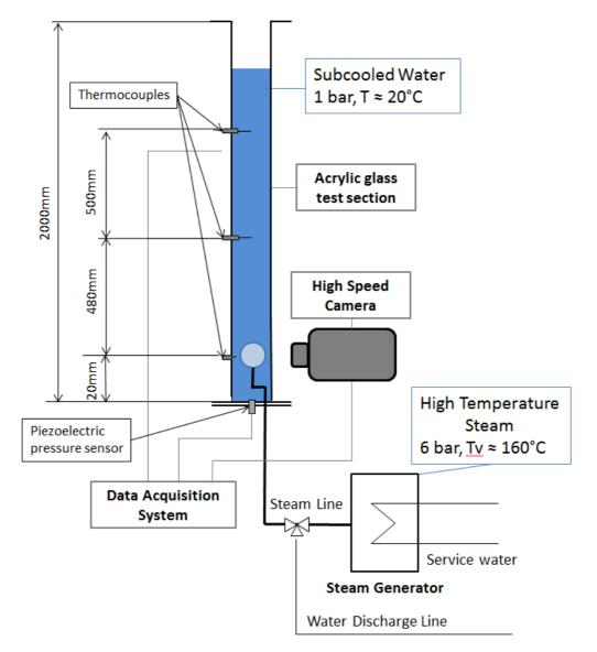
Figure 1: Scheme of the experimental setup of CHUG facility.
