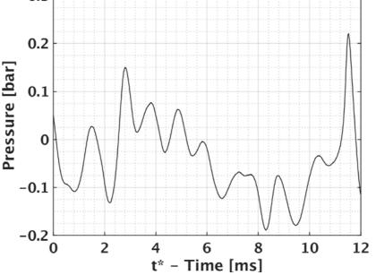
Figure 5: Dynamic measurement of pressure oscillations corresponding to the time interval of the frames of Figure 4: the temperature drift has been corrected.  $t^*$  corresponds to the same time instant of Figure 4.
