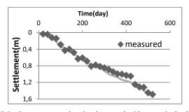
Fig. 8 Settlement versus time implemented with numerical solution
