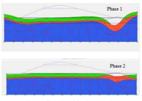
Fig. 4 Deformed mesh in Phase 1 and 2
