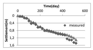
Fig. 7 Settlement versus time implemented with PLASIX
