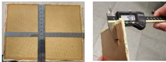
Fig. 23 The dimensions of Kevlar ® plate produced for this study
