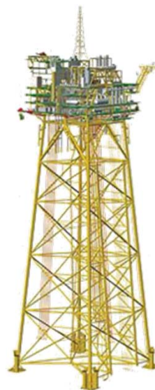
Fig. 1 Typical Jacket Platform (adapted from offshore-technology.com)
