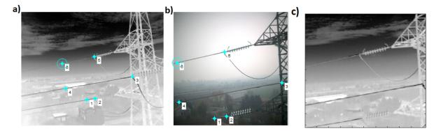
**Figure 6.** Image registration by user-defined control point selection to fuse multiple images from IR and visible cameras. We manually selected the significant feature from both IR and visible images which correspond to each other: (a) Control point selection from IR image. IR image has larger FOV (field of view), so we selected IR image to be registered; (b) Control point selection from Infrared image; (c) IR image after registration.
