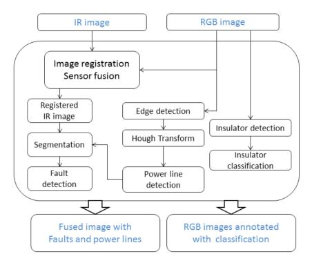
Figure 2. The processing pipeline.
