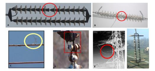
**Figure 1.** A sample of common defects: (**A**) missing plate along the insulator chain; (**B**) missing plate along the (rusted) insulator chain; (**C**) damaged strand of the cable; (**D**) hanging point, damaged by rust; (**E**) cable joints, which are more frequently affected by hot spots; (**F**) a chain of insulators, rusted.
