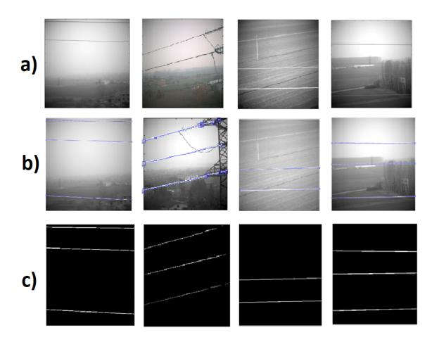
**Figure 9.** Example of power transmission lines with different backgrounds e.g., cluttered, semi-cluttered and with plain background: (a) Power lines on visible image. (b) Detected lines using Hough transform. (c) Segmented power transmission lines.
