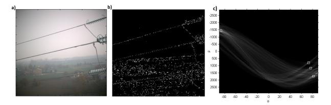
**Figure 8.** (a) Visible image of the tower and power cables; (b) Edges extracted from the visible image using Canny edge detector; (c) Detected peaks with Hough transform, where peaks correspond to the length of the line.  $\rho$  is the perpendicular distance of the peak to the origin and  $\theta$  correspond to the angle. Occurrence of all positive angled peaks correspond to power lines.
