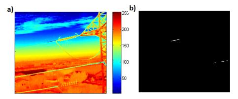
**Figure 11.** (a) Color map of IR image with semi-cluttered background, (b) Obtained hot spot in the power lines. After detecting power lines from visible image, histogram based thresholding on the registered IR image gives expected faults.
