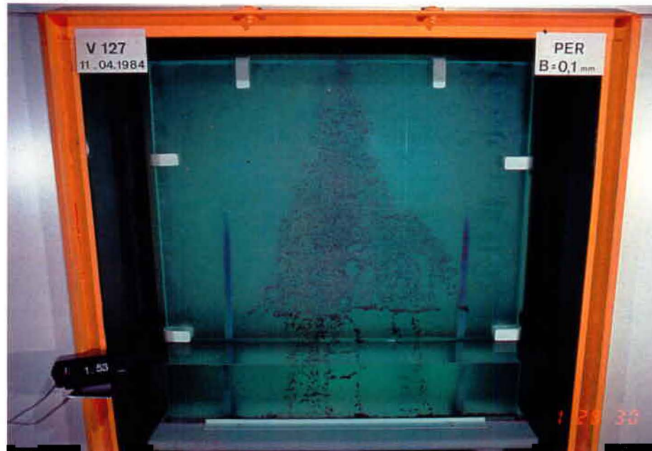
Figure XXII.a. Fracture with an aperture of 0.1 mm, and rough walls initially saturated with water. Water level then lowered. PER then applied at 1.3 mL/min. Water remaining on fracture walls affected distribution of PER.
