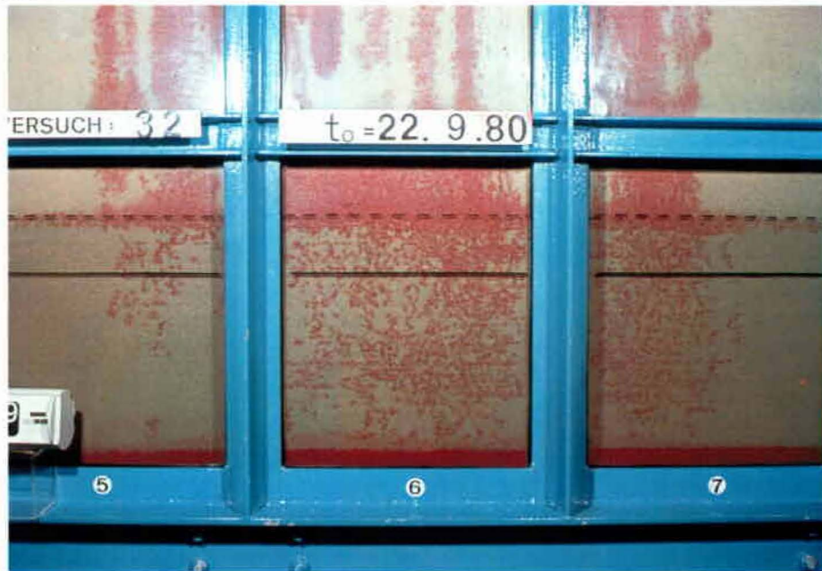
Figure X.a. Sheet-like spill of 36.3 L of PER. View of spill above the capillary fringe.
