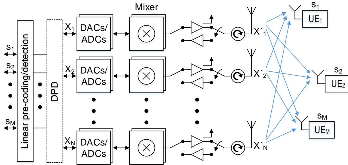
Digital beamforming/mMIMO is used at sub 6GHz frequency bands today
