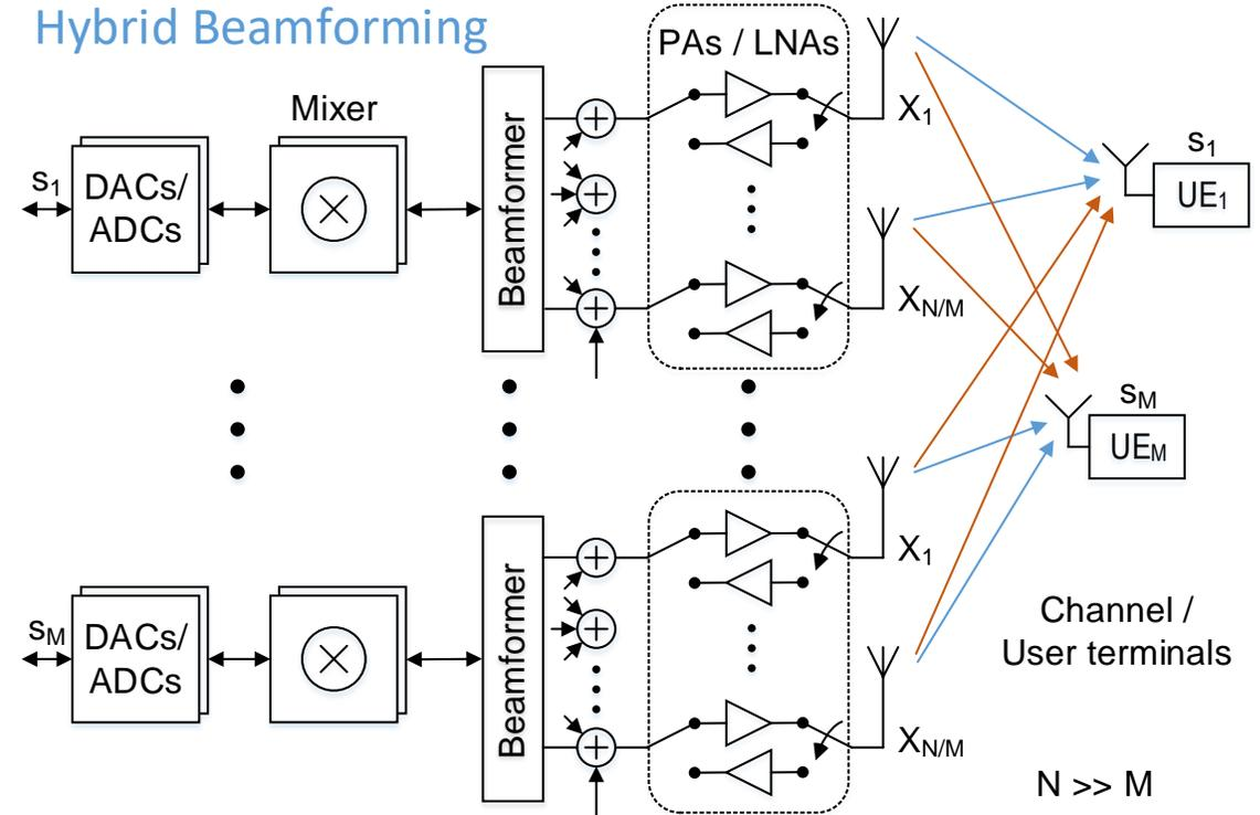
Hybrid beamforming is used at mm-Wave frequency bands today
