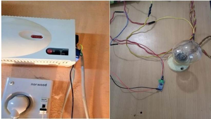
Fig. 7. sensors attached to an air conditioner and bulb
