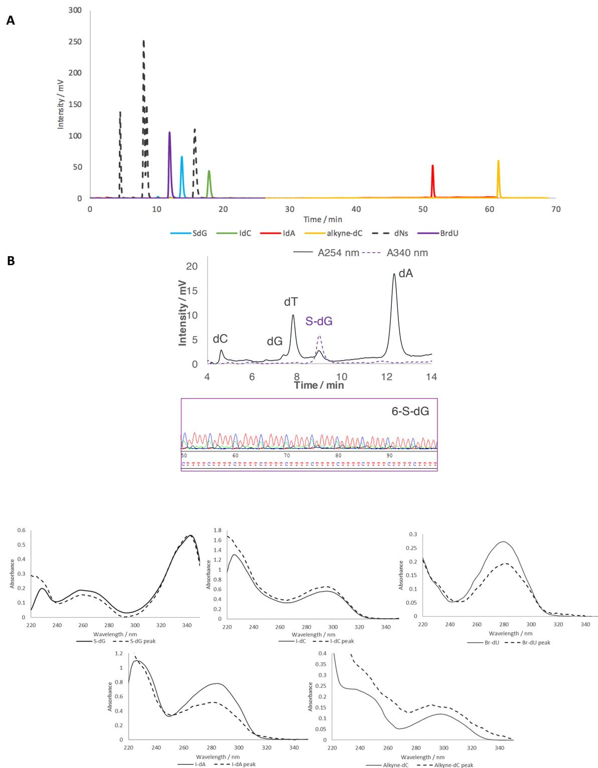
Standards of each deoxynucleotide (dN) were used to determine HPLC elution times, shown as a HPLC trace (**A**) using the method described, see Supplementary Table 1. To determine extinction coefficients, a known mass of each dN was measured and prepared to a known concentration. Each dN was then analysed by
