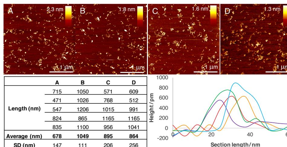
AFM images (A-D) of 5-(octadiynyl)-dCTP, a table of the analysed lengths and a selection of perpendicular height scans.
