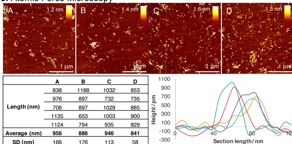
AFM images (A-D) of 5-I-dC-DNA, a table of the analysed lengths and a selection of perpendicular height scans.
