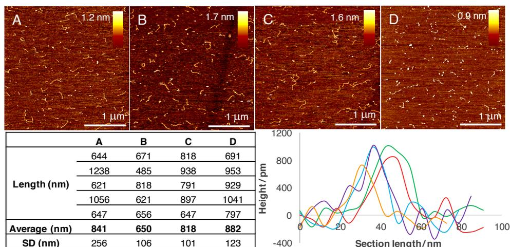
AFM images (A-D) of 7-deaza-7-I-dA-DNA, a table of the analysed lengths and a selection of perpendicular height scans.
