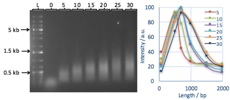
Agarose gel of Hg-dC-modified DNA extension products after 5, 10, 15, 20, 25 and 30 cycles is shown. Extension was performed with  $[A_4G]_4/[CT_4]_4$  and shows successful DNA extension.
