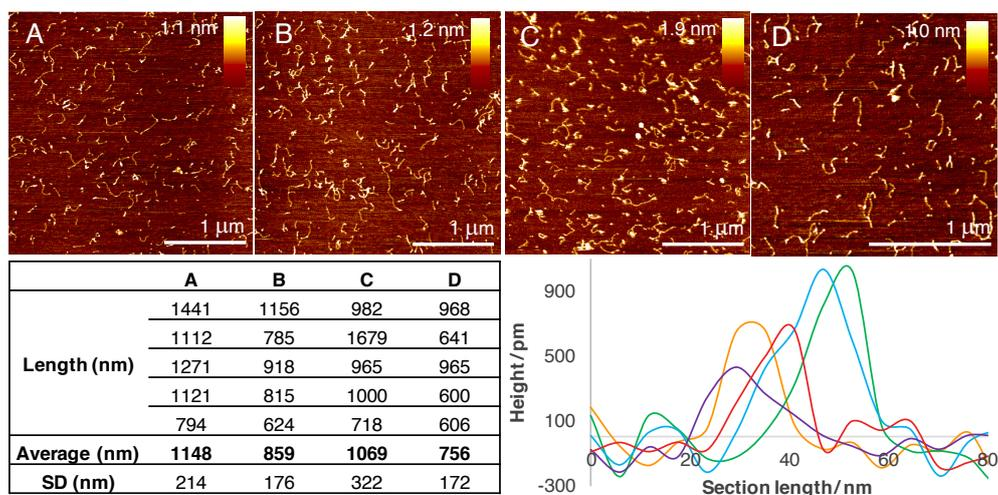
AFM images (A-D) of 5-Br-dU-DNA, a table of the analysed lengths and a selection of perpendicular height scans.
