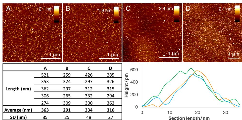
AFM images (A-D) of 6-S-dG-DNA, a table of the analysed lengths and a selection of perpendicular height scans.
