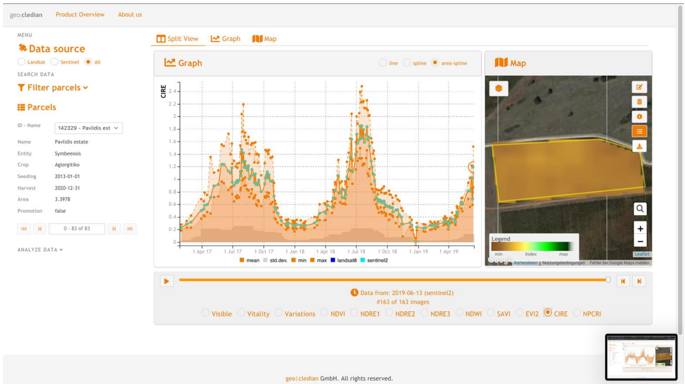
Figure 6: A Sentinel-2 CI-RE time series for 2017 - 2019 for a parcel of the Pavlidis estate, Greece showing also the NDVI image for 13th June 2019. The Chlorophyll Index-Red Edge (CI-RE) is reported to be highly correlated with canopy Chlorophyll and Nitrogen contents.
