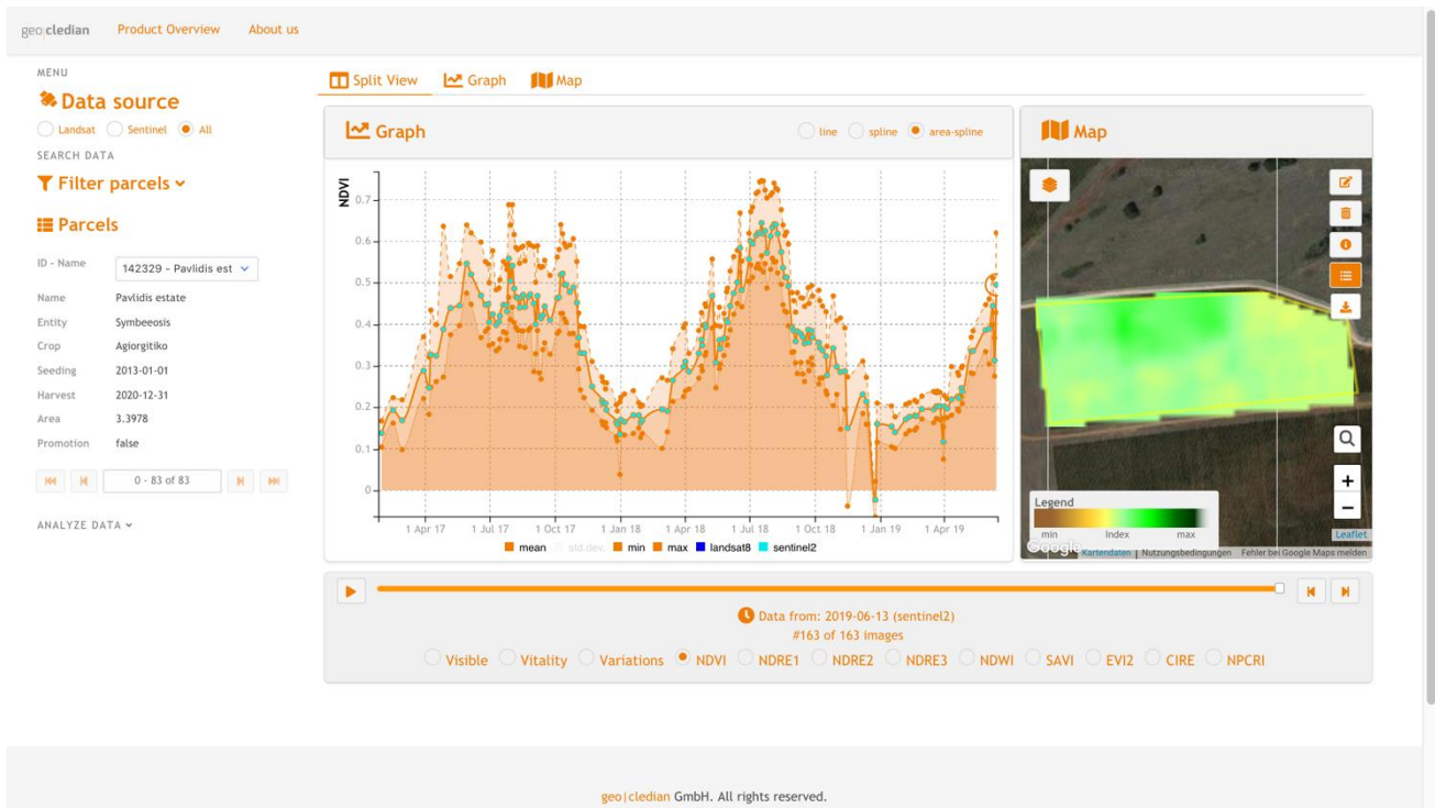
Figure 4: A Sentinel-2 NDVI time series for 2017 - 2019 for a parcel of the Pavlidis estate, Greece showing also the NDVI image for 13th June 2019.
