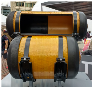
700 bar \text{cH}_2 tanks onboard Toyota Mirai
