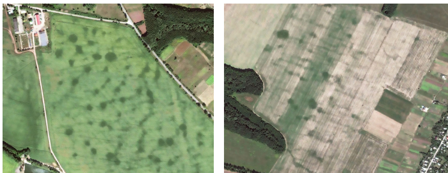
Fig. 4.34. Examples of suffosion subsidences in Kyiv Region; according to satellite images of Stayky Village, Kaharlytskyi District (a) and Vytachiv Village, Obukhivskyi District (b).
