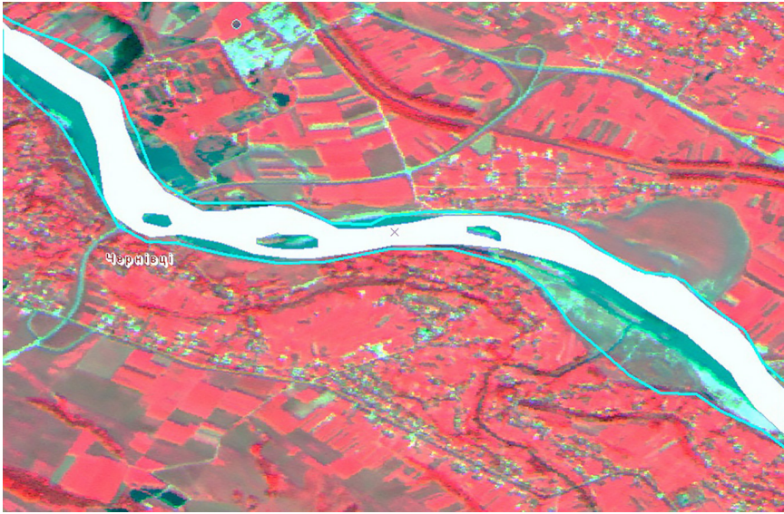
Fig. 4.107. RapidEye image as of July 27, 2008 — end-stage freshet on Prut River (blue contour — maximum overflow of the river; white contour — river bed prior to freshet start, at the beginning of July). Source: archival data of “GIS Analyst Center”, LLC
