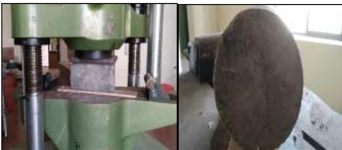
Fig. 5. (a) Split tensile strength test and (b) Cracked cylinder after split tensile strength test
