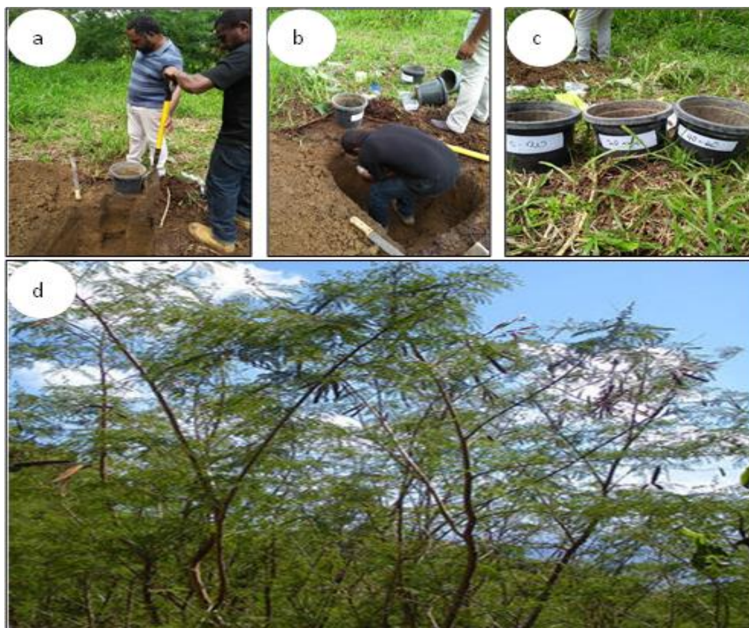
Figure 2. (a) Digging 60 cm piths, (b) sampling, (c) collecting samples in labeled buckets, and (d) sample photo showing the density of the legume trees of the study site
