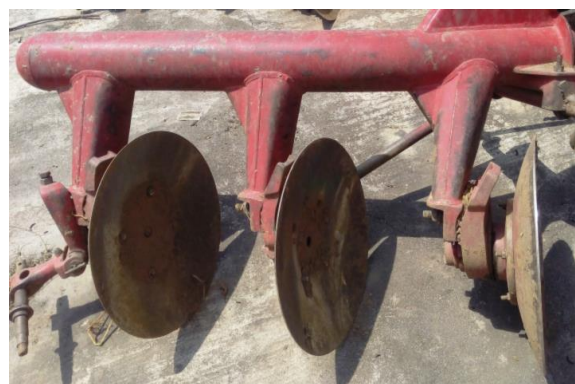
14. Disc plough with improper adjustments of working organs and depth.
