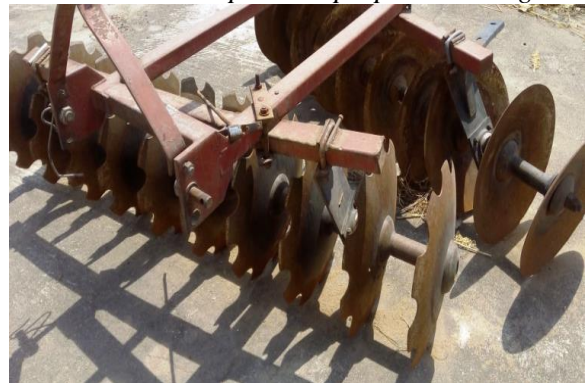
12. Disc Harrow with improper adjustments of working organs and depth
