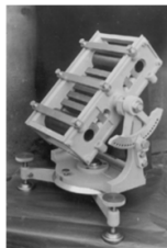
The CR telescope used by Bruno Rossi during the expedition in Eritrea
