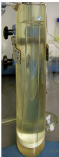
Figure 3.2.: Double-walled gelation column, filled with silicone oil.
