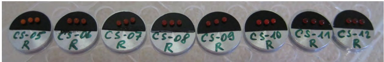
Figure 3.10.: Microspheres prepared for SEM/EDX investigations.
