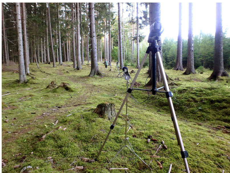
Plate 1. Recording setup with singer and three camcorders/microphones at 1 meter, 11 meters and 22 meters from the singer. Photo by first author.
