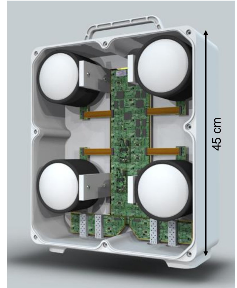
A mock-up for 8x8 LoS-MIMO at D-band (target at 200m hop distance)
