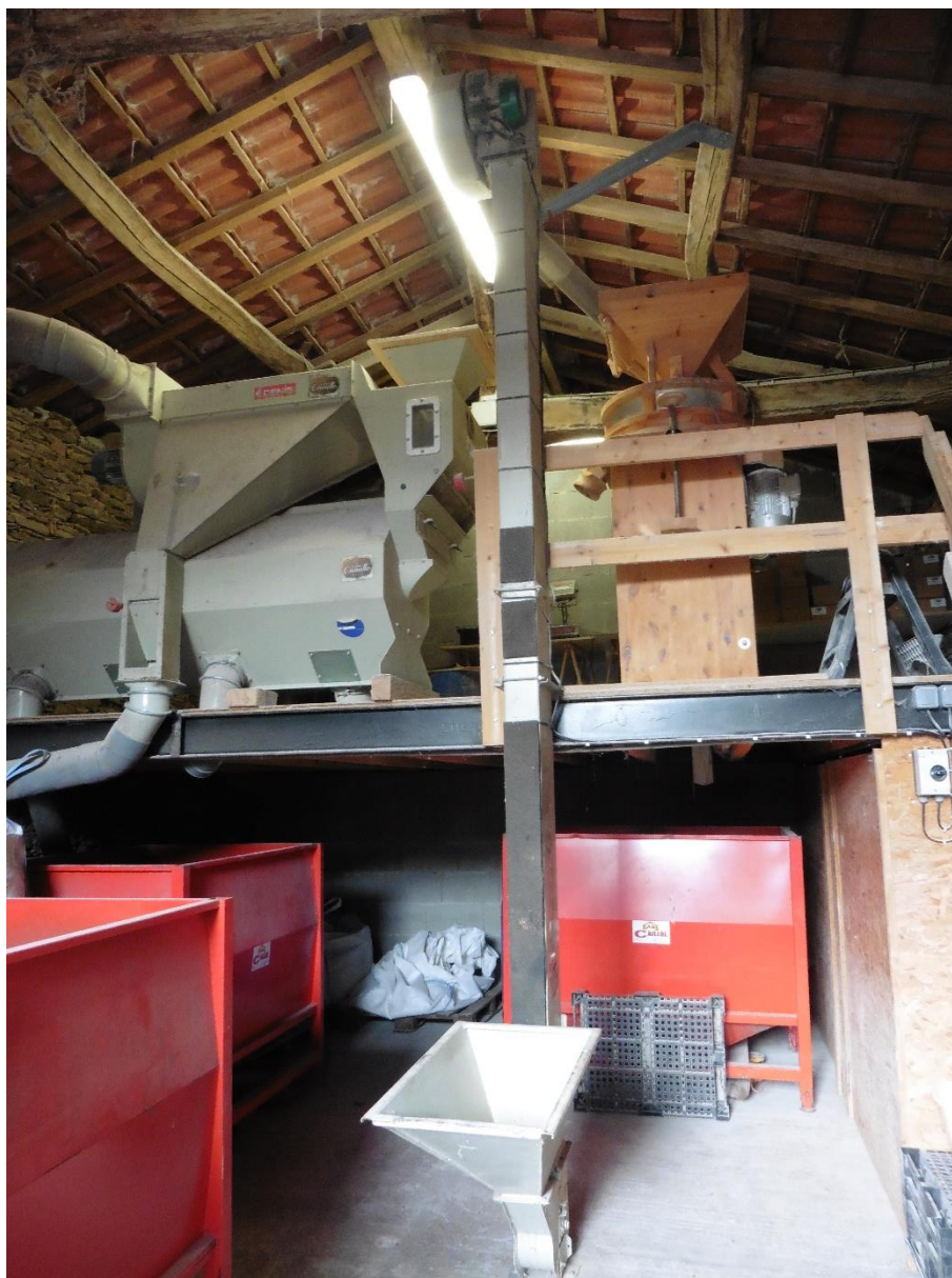
The elevator (in the middle), the mechanical screener (top left) and the mill (top right)
