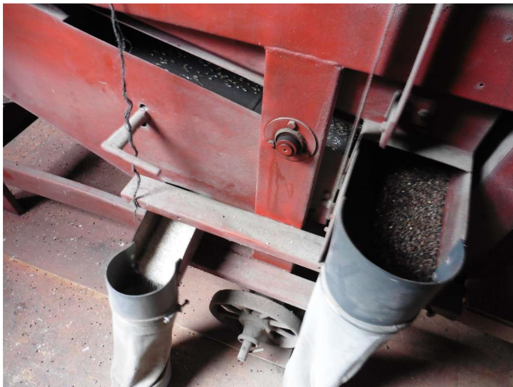
The mechanical screening using moving grids for the second screening after dehulling
