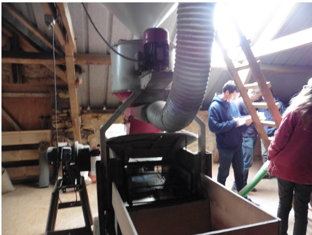
The winnowing machine below (Tarare) used for the first wind screening
