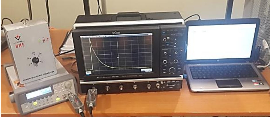
Figure 2. Implemented Reference PD measuring system
