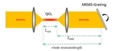
Figure 1. Schematics of a (MOEMS) EC-QCL setup in Littrow configuration.
