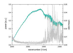
Figure 4. Intensity plots for 30 periods in pulsed mode for a scanning MOEMS grating following a triangular trajectory with 10 Hz scan frequency. The data was smoothed by using a 20 points running average. For wavelength larger than 2300 cm<sup>-1</sup> strong CO<sub>2</sub> absorptions are observed, which also cause a dramatic increase in noise, which is plotted in the same graph.
