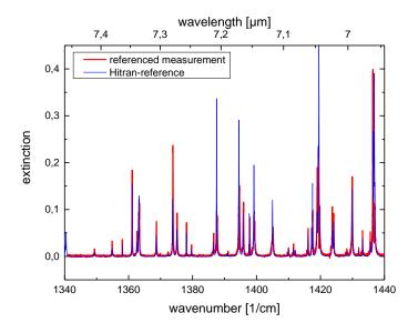
Figure 8. Demonstration of a high-resolution transmission spectrum of water vapor obtained with a fast-scanning MOEMS EC-QCL on a linear positioner.
