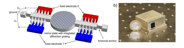
Figure 2. a) Schematics of the quasi-static MOEMS micromirror with integrated diffraction grating. The static electrodes of the staggered vertical comb drives are highlighted in red and blue. The (static) potentials are applied to those.<sup>11</sup> b) Picture of the integrated quasi-static MOEMS EC-QCL module.
