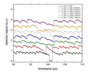
Figure 6. Intensity vs. time (-> grating angle) during a MOEMS scan for various length settings of the external resonator, demonstrating regular (black line) behavior with steps of identical length, as well as hardly predictable situations (e.g. green line). Note that the "dip" in intensity at ~101  $\mu$ s is due to atmospheric water absorption between laser and detector and not a feature of the laser itself.
