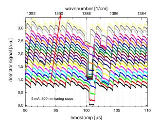
Figure 7. Principle of high spectral resolution by combining several scans with different length / current settings. The wavelength is constant in between mode hops ( $\sim$ 1 µs in this example) and shifted slightly in every new trace by length / current adaption.
