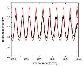
Figure 5. The transmission measurement through a GaAs wafer shows a pronounced etalon effect. In black are the results from the measurement with the laser operated in pulsed mode and the MOEMS grating running at a 10 Hz repetition rate for forward and backward motion. For the simulation we assume a refractive index of n=3.2 and a thickness of 114  $\mu$ m. The assumed linewidth is zero.
