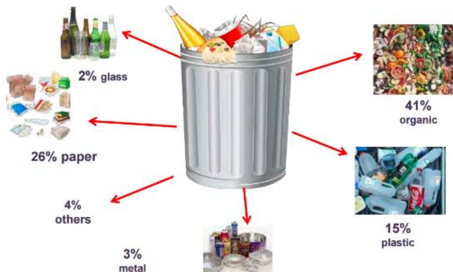
Characterization of waste in Cyprus: main streams are organic fraction, paper and cardboard, plastic (source: green-dot Cyprus, 2017)
