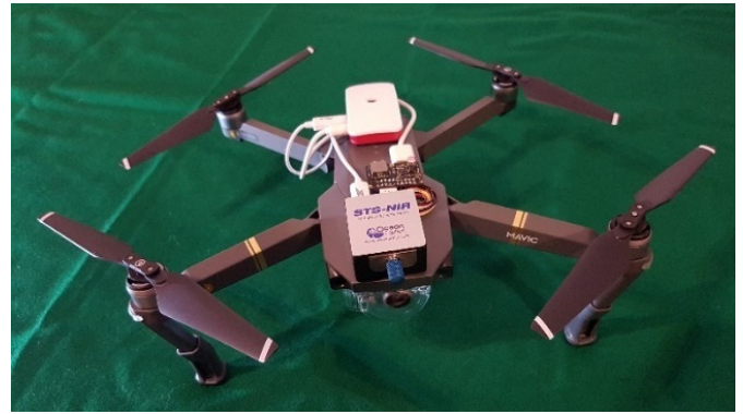
Fig. 2 First version of the fire detection sensor on RASPI 3 (a) and the final one on PI-Zero W (b).
