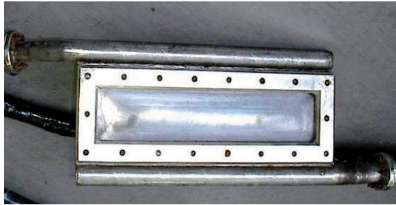
Fig. 2.29. Electron beam–X-rays converter (tantalum – 0.5 mm, H 2 O – 20 mm, steel – 0.8 mm)
