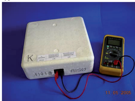
Fig. 4.2. Calorimetric dosimeters: graphite (A) and polystyrene (B) used for electron beam related measurements
