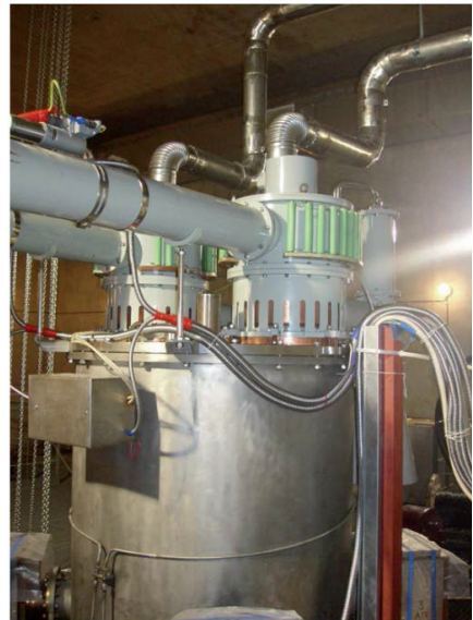
Fig. 7.8. RF electron accelerator type ILU 10: 1 – vacuum envelope, 2 – resonator, 3 – focusing coil, 4 – ion pump, 5 – electron gun, 6 – scanner, 7 – coupling loop support, 8 – vacuum capacitor, 9 – RF generators
