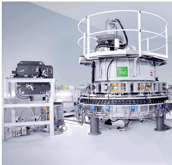
Fig. 7.9. RF electron accelerator Rhodotron TT200 type: 1 – vacuum envelope, 2 – electron gun, 3 – RF tetrode amplifier, 4 – deflecting electromagnet, 5 – bending electromagnet
