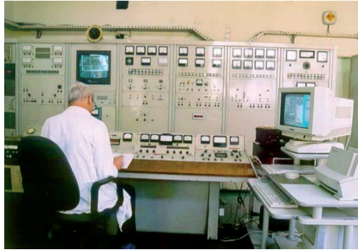
Fig. 3.44. Control room of LAE 13/9 electron accelerator and data collection system for radiation sterilization process
