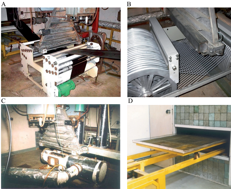
Fig. 3.35. Pilot plant facility arrangement with different irradiated product transport systems: A – heat-shrinkable tapes, B – electrical wires and cables, C – gaseous pollutants removal, D – close loop conveyor
