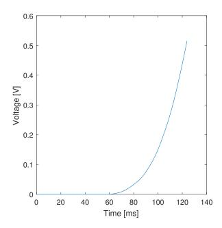
Figure 6.3. Coil's resistive voltage as a function of time.
