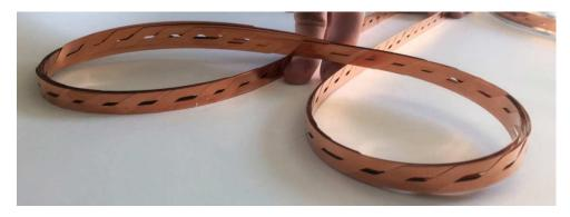
Figure 2.8. Photograph of a Roebel cable. Figure from [60].
