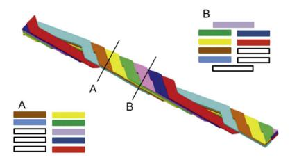
*Figure 2.6.* Structure of a Roebel cable. Figure from [19].
