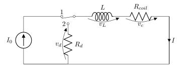
Figure 3.5. Circuit diagram of the energy extraction system.
