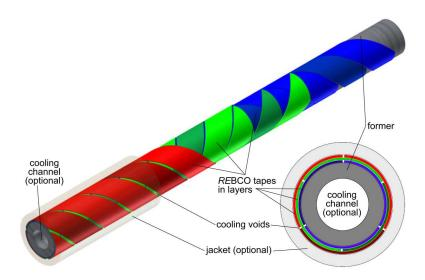
*Figure 2.9.* Depiction of a HTS tape based CORC cable. Figure from [3].
