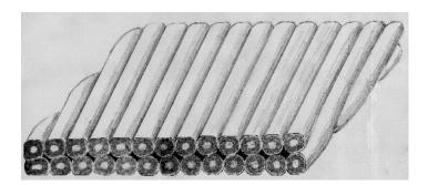
*Figure 2.4.* Geometry of Rutherford-cable. Figure from [65].
