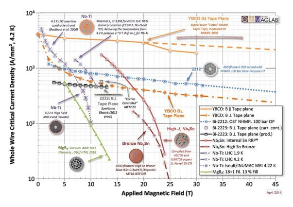
Figure 2.1. Engineering current density as a function of applied magnetic field for present conductor types. Figure by MagLab [32]
