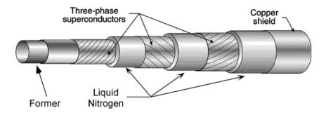
*Figure 2.11.* Three-phase superconducting powercable. Figure from [20].
