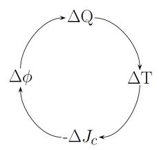
Figure 3.3. Illustration of a quench chain reaction Figure from [21]...
