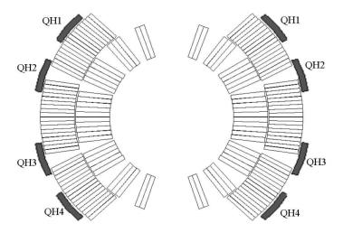
Figure 3.6. Four quench heater circuits are implemented on the LHC main dipole magnet's most outer winding layer. Figure from [44].
