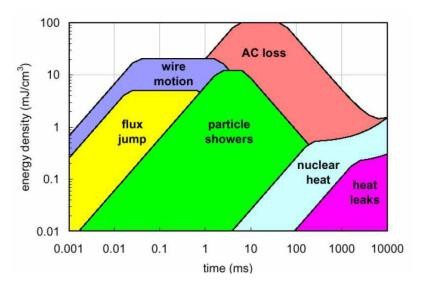
Figure 3.1. Depiction of superconductor disturbance spectrum in an accelerator magnet. Figure from [6].
