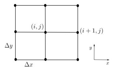
Figure 4.4. Two-dimensional discretization for FDM.
