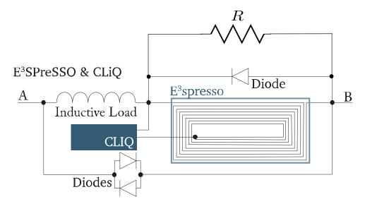
Figure 3.8. A sketch of  $E^3$ SPreSSO unit with CLIQ-activator. Figure from [61].
