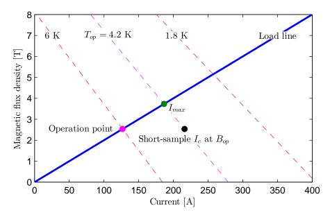
Figure 3.4. Illustration of magnet's load line (solid line) and critical current characteristics at different temperatures (dashed line).
