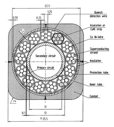
Figure 2.5. Cross-section of the POLO conductor. Figure from [24].
