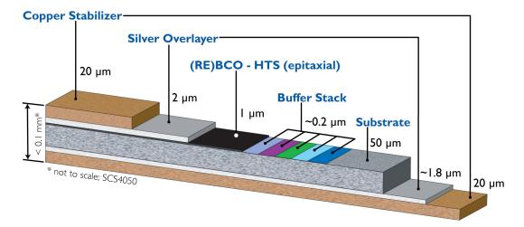
Figure 2.3. Structure of a REBCO tape. Figure from [58].
