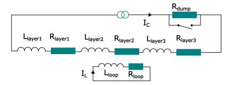
Figure 3.9. A circuit diagram illustrating the ICED concept. Figure from [40].
