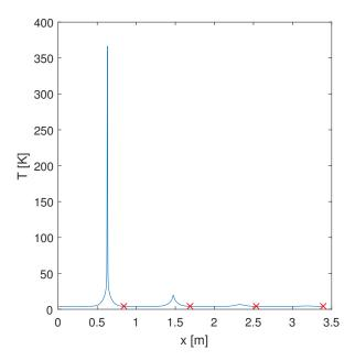
**Figure 6.5**. Temperature distribution along the coil length (x-axis), when hot spot temperature is at its maximum. The change of cable turn from previous to next one is marked with red crosses. The winding starts (x=0) from the middle of the straight part of the coil from the innermost cable turn.
