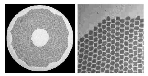
Figure 2.2. Photo of cross-section of a NbTi conductor. Figure from [65].
