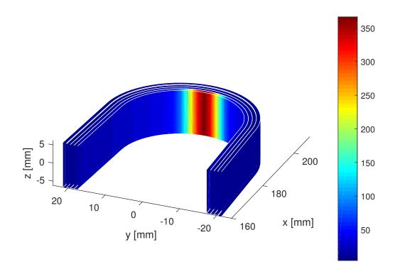
**Figure 6.7**. Temperature distribution in 3-D. Temperature colorbar on the right hand side in the figure is in Kelvins. The coil was quenched at the end of it in the first cable turn.  $I_{op} = 6 \text{ kA}$ ,  $t_{del} = 30 \text{ ms}$ ,  $V_{det} = 100 \text{ mV}$ .
