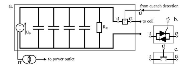
**Figure 3.7**. A schematic of CLIQ unit's circuit diagram (a.). The trigger box, T, can be either a diode-thyristor anti-parallel connection (b.), or an electronic switch (c.). Figure from [44].
