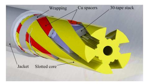
Figure 2.10. Twisted-stack cable geometry. Figure from [9].
