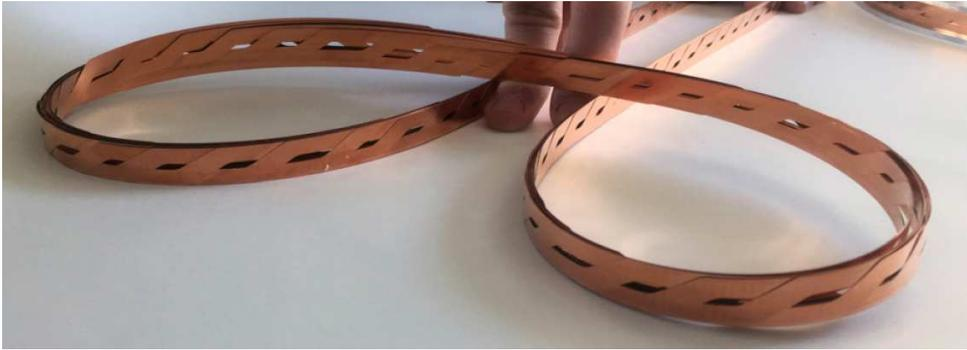
**Figure 2.8.** Photograph of a Roebel cable. Figure from [60].
