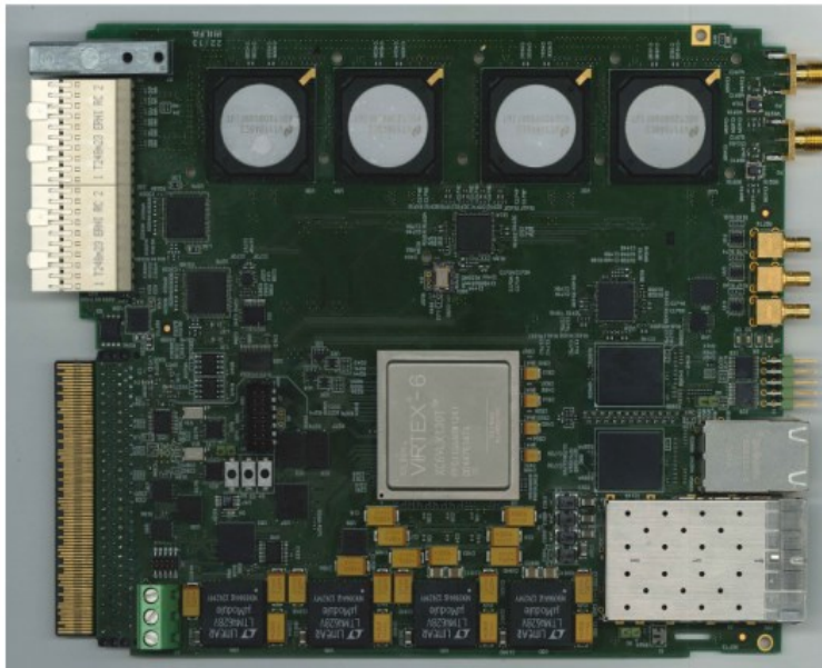
Figure F.6 Photo of DAMC-DS800 MTCA.4 Fast Digitizer. The future electronics will be slightly different from this picture. (Courtesy of Samer Bou Habib)
