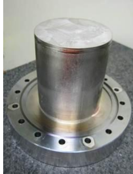
(b) Niobium sample fully assembled
