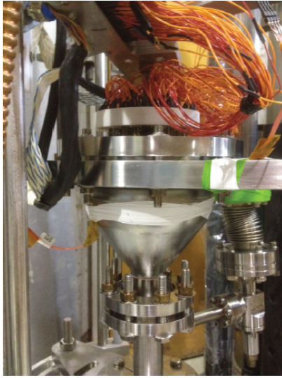
Figure 3.1: Photo and results of the TE host cavity at Cornell [46, 47]. The surface resistance of the sample can be measured in an integral RF measurement. The thermometry system, mounted to the backside of the sample (orange cables), can be used to detect local hot spots. Peak fields of over 100 mT have been reached with this setup
