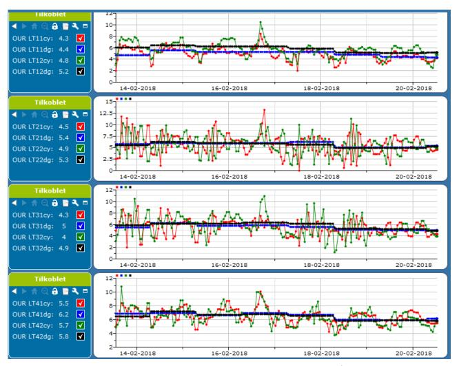
Figure 11 - OUR Oxygen Uptake Rate calculated in 8 aeration tanks (g  $O_2/m^3$ /hour). The graph is from the STARpro control system and shows two curves for each aeration tank. The ones with much variation (..cy) is based on cycles calculations (nitrification+ denitrification) whereas the more stable curves (..dg) is based on diurnal averages.
