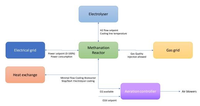
Figure 19 - Overviwe of the dommunication interfaces necessary for a full integration of the biomethanation plant to the Wastewater Treatment plant.
