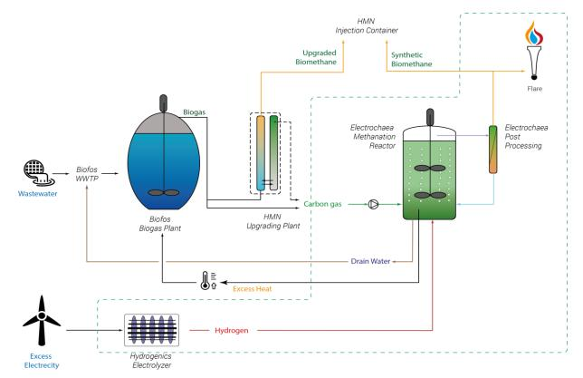
Figure 4 - General layout and integration of the BioCat reactor. Electrochaea perimeter is delimited by the green dashed line, future upgrading plant in black-dashed line.
