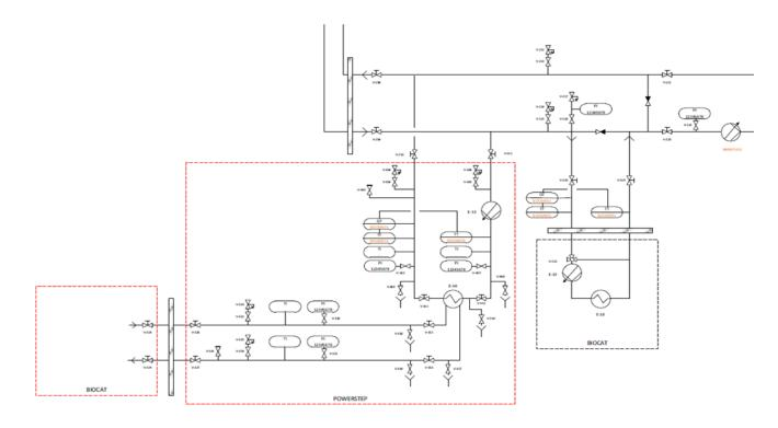
Figure 14- Modification of the heating/cooling system to recover heat from the electrolyzer.
