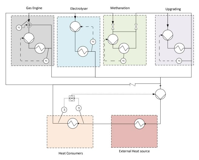
Figure 20 - Simplified PFID of the heat exchange between Biofos heat consumers and the three intermittent heat sources (gas engine, methanation reactor and electrolyzer, the biogas upgrading plant)
