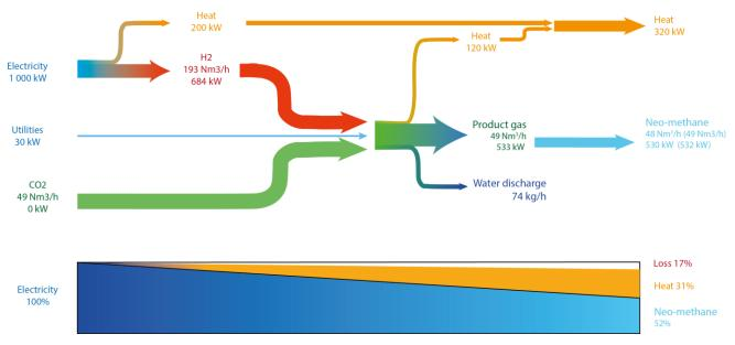
Figure 7 - Mass and Energy balance with CO2 as primary carbon source
