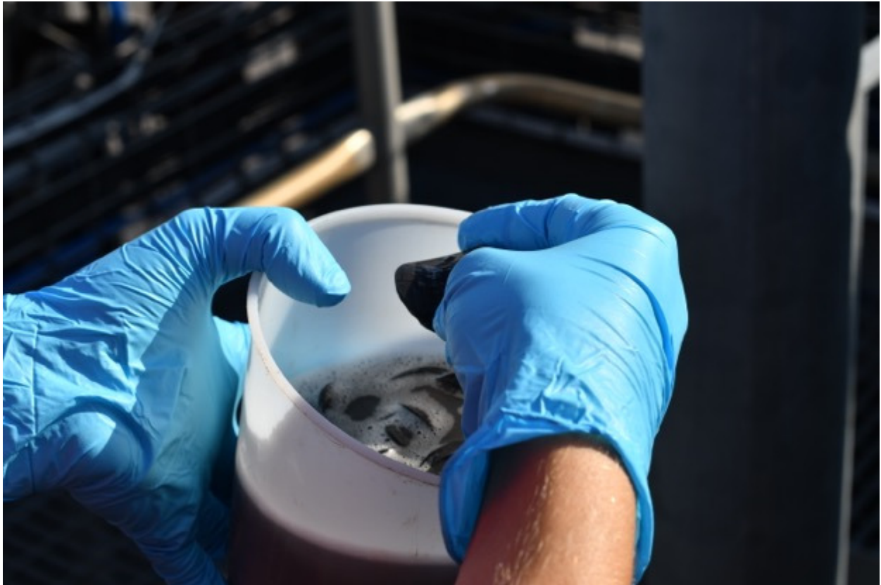
Figure 9: Chips for Main stream annamox reactor in Sjölunda Case Study Site 2
