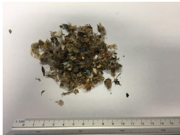
Figure 15: Light material in the form of relatively coarse plastic fragments. These solids resulted from the co-digestion of food-waste at WWTP Altenrhein (results by SUSTEC BV)
