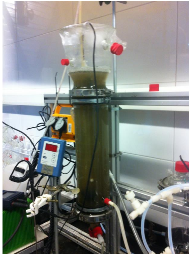
Figure 16: Lab-scale tests for removing CO 2 from sludge liquids by stripping with air (trials by SUS-TEC BV)
