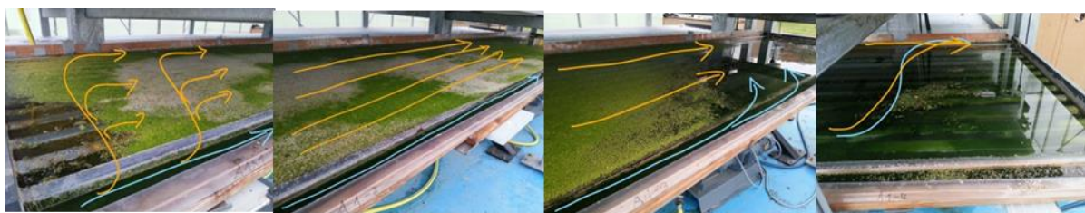
Figure 36: Flow behaviour of the filter as it is (blue) and how it should be (orange)
