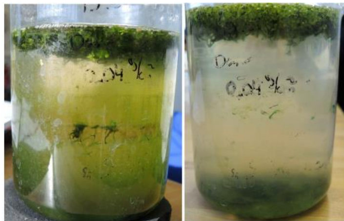
Figure 23: Formation of submerged algae in beaker with duckweed mat density of 0.05 \text{ g}\cdot\text{m}^{-2} without side cover (left picture; 16.02.2017) and with side cover (right picture; 10.03.2017)
