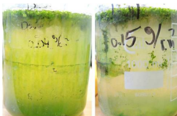
Figure 20: Comparison of algae formation at different mat densities from 03.03.-09.03.2017: Left beaker: Mat density 0.05 g·cm -2 ; Right beaker: Mat density 0.15 g·cm -2
