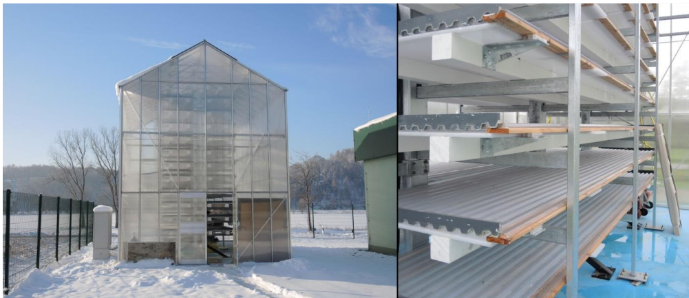
Figure 6 Left: Front view of Greenhouse containing the APS duckweed plant; Right: duckweed plant trays of the APS system inside the greenhouse
